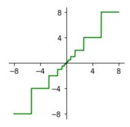
Figure 2: Log-quantization step function.
